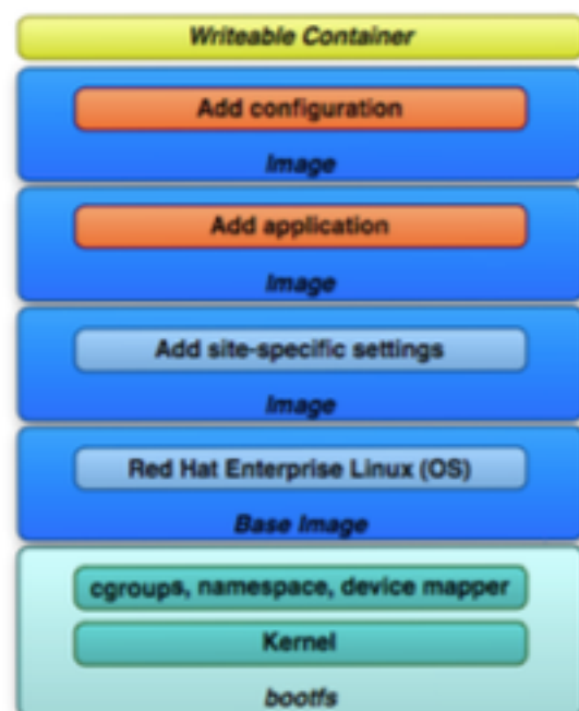
Figure 4: The layers of the Docker file system
